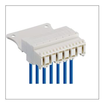
RAST 5 connector for indirect mating, with screw terminal, with lift clamp with protection against misplacing, with test holes and interior locking, consecutive placement without loss of pitch, cable departure on side of lock, with handle latch
